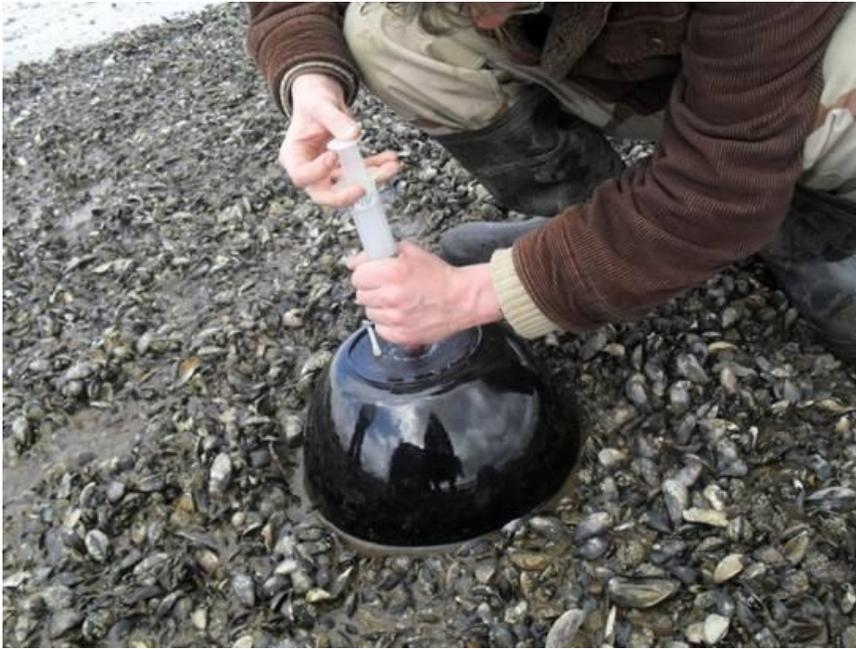
**Figure 14.** Sample being extracted from a gas collection chamber situated on a mussel-bed.
