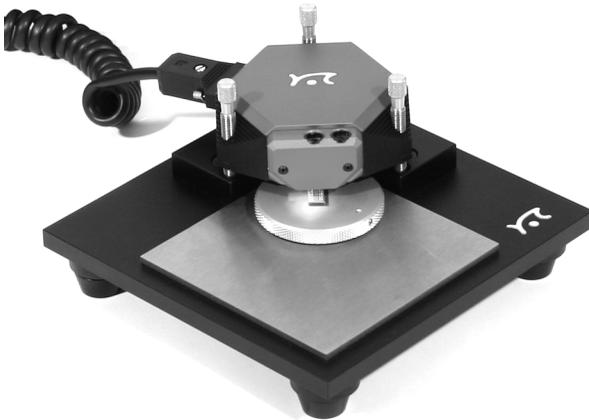
*easyScan 2 AFM Scan head on the Sample Stage*
