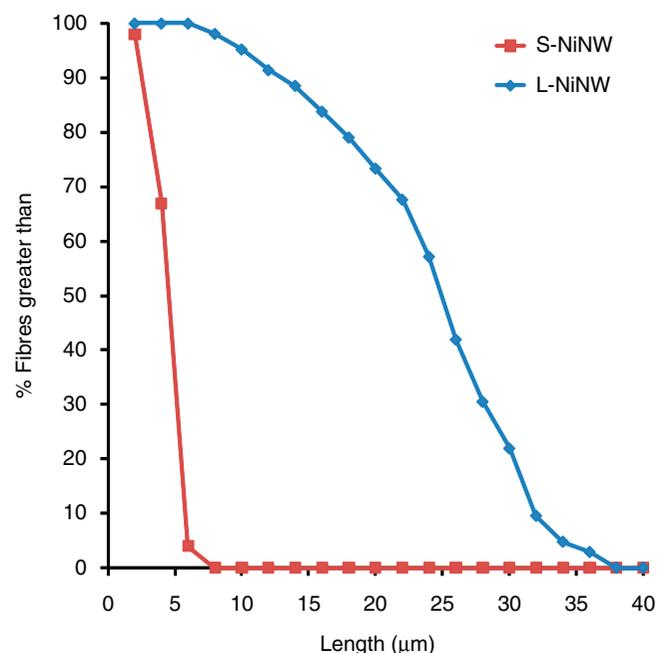
Figure 3. Nickel nanowire size distribution. Size distribution was performed by measurement of a minimum of 100 fibres imaged under scanning electron microscopy (SEM, Carl Zeiss Ultra Plus, UK).
