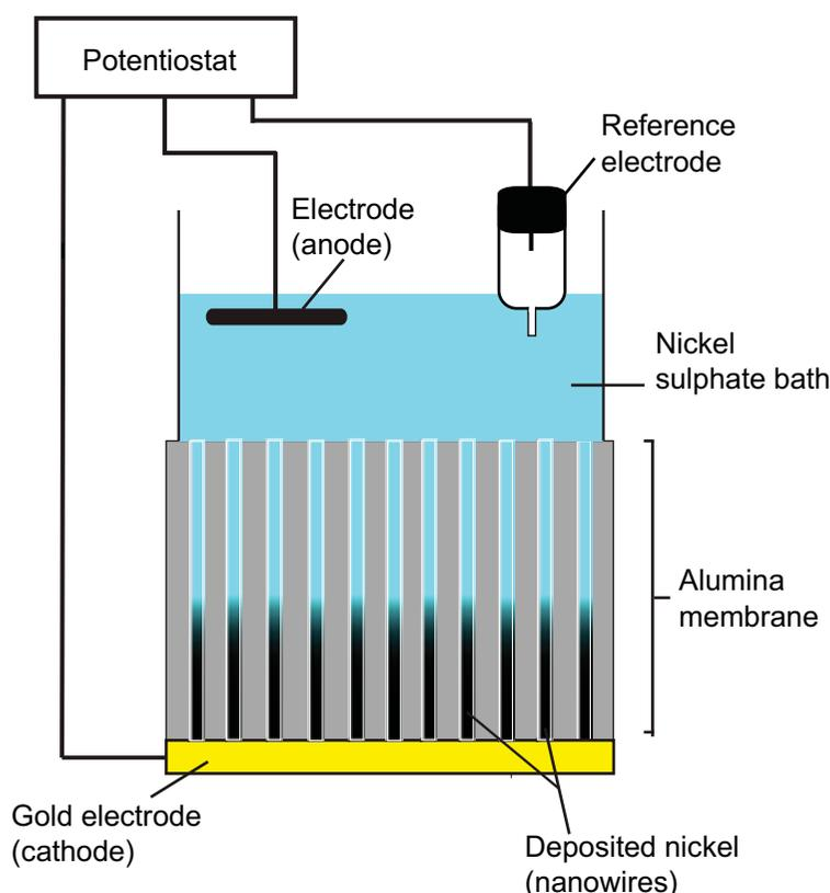
Figure 1. Diagram of nickel nanowire synthesis. The typical template mechanism for the production of nickel (and other electrically conductive material) nanowires is shown (adapted from Cao & Liu 2008).
