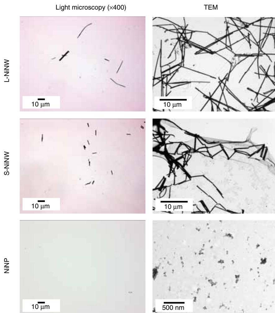
Figure 2. Morphological structure of nickel nanowires (NiNW) and nickel nanoparticles (NiNP). Brightfield images of nickel based nanoparticles were taken at  $\times 400$  magnification in glycerol after dispersion in  $\text{dH}_2\text{O}$  (left hand panel). TEM images were taken for NiNP dispersed in  $\text{dH}_2\text{O}$  and deposited onto formvar coated TEM grids (0.5  $\mu\text{g}$ ) prior to imaging. (Right hand panel) (Please note the different scale bar between TEM of NiNW and NiNP).
