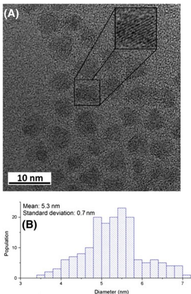
**FIGURE 1** (A) TEM image and (B) size distribution diagram of oleylamine-stabilized ZnS:Mn QDs in chloroform. The insert in (a) shows HR TEM image of QDs
