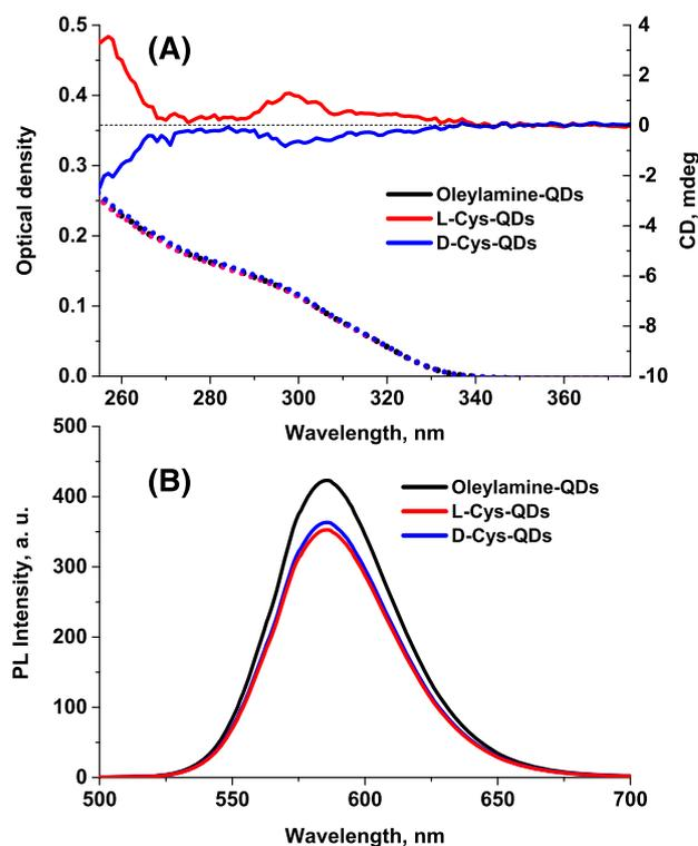
**FIGURE 2** Optical properties of oleylamine-QDs before (in chloroform, black curve) and after ligand exchange with L- and DCys (in water, red and blue curves, respectively): (A) UV-vis and CD spectra, (B) PL spectra. QDs concentration was 3  $\mu\text{M}$  in samples for CD measurements and 0.3  $\mu\text{M}$  in samples for UV-vis and PL measurements
