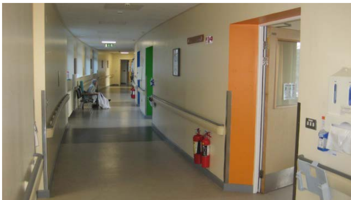
Figure 4.23 – Corridor in Rowan ward showing colour contrast to skirting and accent colours to patient rooms
