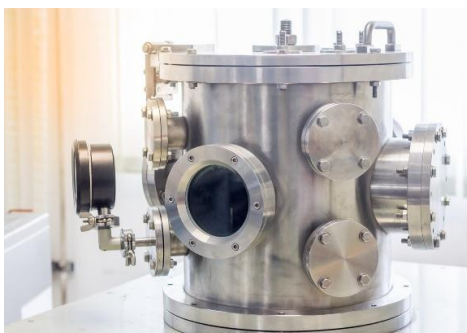
Figure 1. Example of a typical steel vacuum chamber with multiple access ports.
