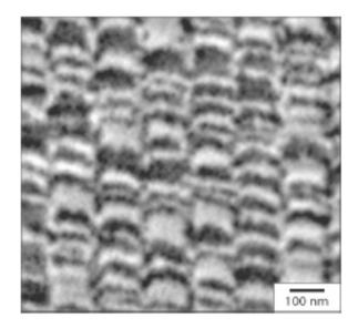
Perpendicular tracks on a hard disc imaged by high-resolution magnetic force microscopy. The width of the tracts is determined by the width of the write head. The recording density here is 300 bits  $\mu$ m<sup>-2</sup> or 250 Gbit/square inch. (Courtesy of Nanoscan AG.)
