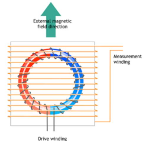
Fluxgates are bulky but sensitive, reliable and impervious to radiation. Used, for example, in space.
