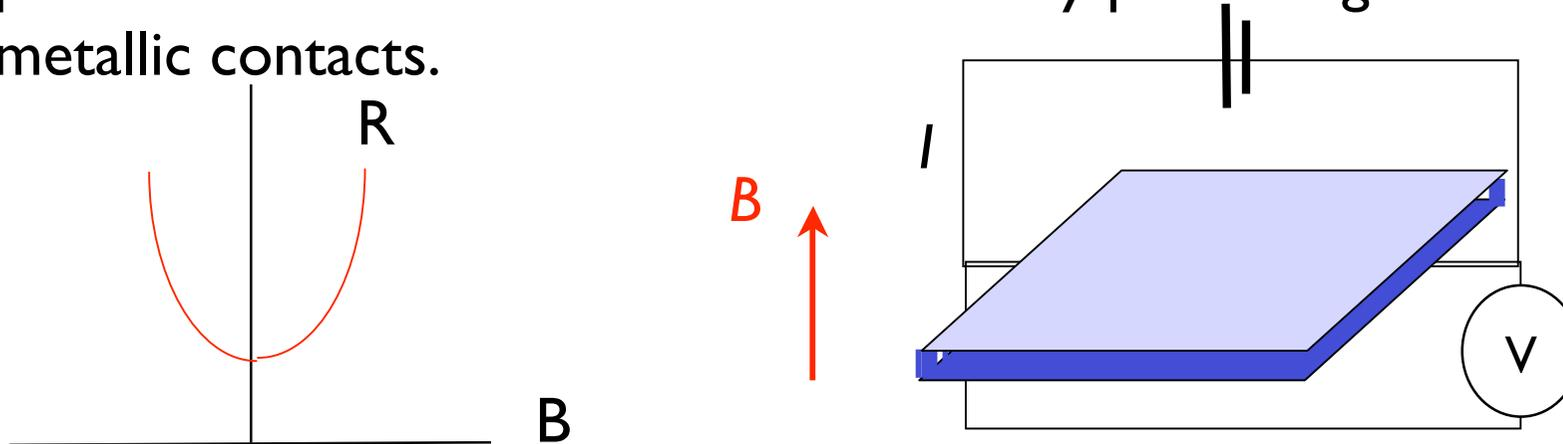
The sensors are nonlinear, two-terminal devices providing a good response in large fields. They are used as position sensors in brushless dc permanent magnet motors.
