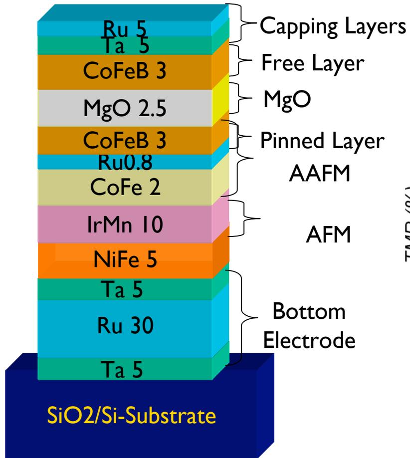
Magnetoresistance is > 100%, 10 times as great as for GMR spin valves
