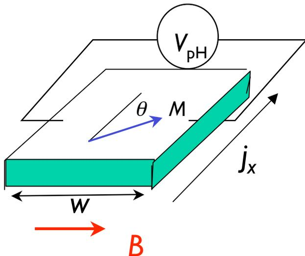
$$E_{\parallel} = \rho_{\parallel} j_x \cos \theta \quad E_{\perp} = \rho_{\perp} j_x \sin \theta$$
