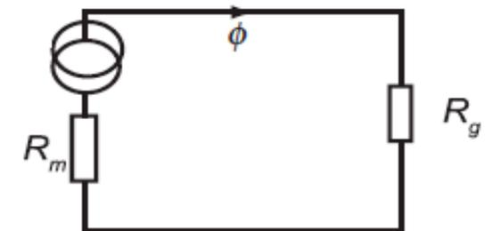
**Figure** A simple magnetic circuit, and its electrical equivalent, with and without losses.
