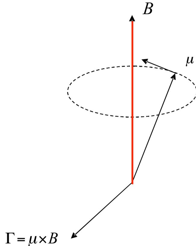
Torque creates precession at the Larmor frequency  $f_L = \gamma B / 2\pi$
