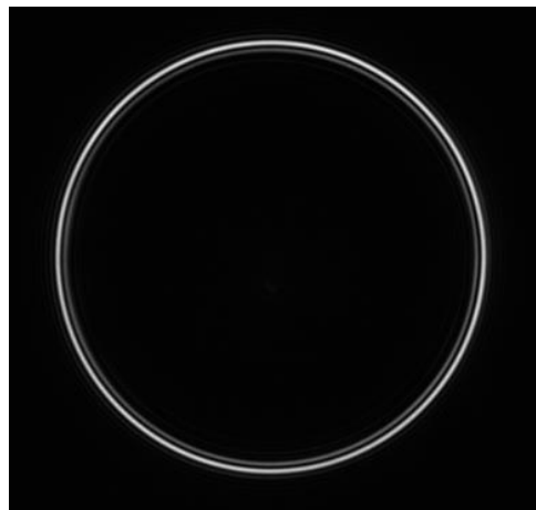
Figure 3. Photograph of a magnified image of the double-ring formed at the focal image plane by internal conical diffraction of a Gaussian laser beam [7].
