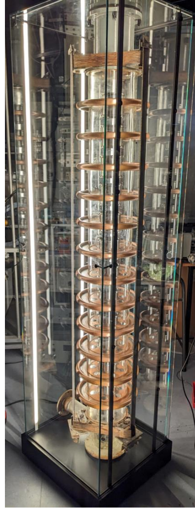
The accelerator tube with the specially shaped metal conductor Einzel lenses.
