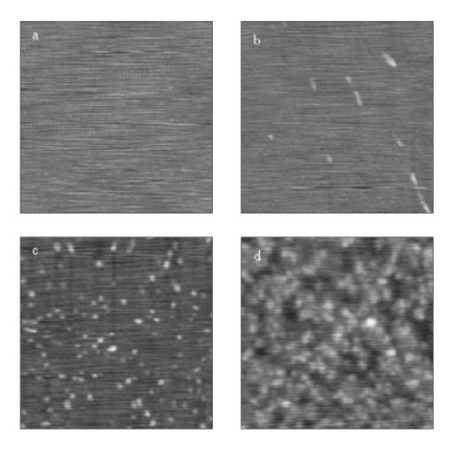
Figure 5: Interferon  $\alpha$ -2a adsorbed from citrate buffer (pH 5) onto mica at a concentration of (a) 4.75 µg/mL and (b) 9.5 µg/mL. Topography images (size: 500 x 500 nm, grey scale: 1.6 nm) were taken in air.
