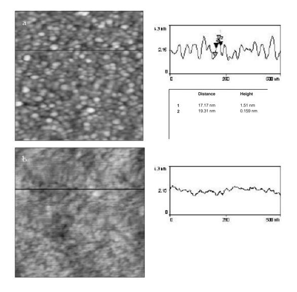
**Figure 7: Enlargement of the size of a topographic feature with radius r when imaged with an AFM-tip with radius R.** The observed width W of the molecule can be calculated by using the following equation:
