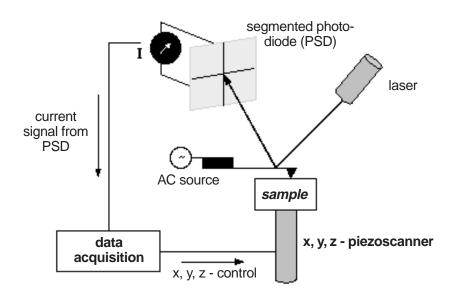
phase when the apex of the tip is approaching the sample surface, topographical data can be detected in a very sensitive and gentle way. AFM allows forces to be measured in the piconewton range and it enables, at the same time, study of biological specimens *in situ* in a physiological environment (2-4).
