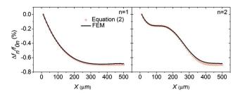
Fig. 5 Modelling of hyphal growth along the length of a 7  $\mu$ m thick cantilever. Plots are shown for the fundamental and second resonance modes. Calculated frequency shifts using both methods agree. As is observed experimentally there are no negative frequency shifts observed in regions of the cantilever where vibrational amplitude is small.
