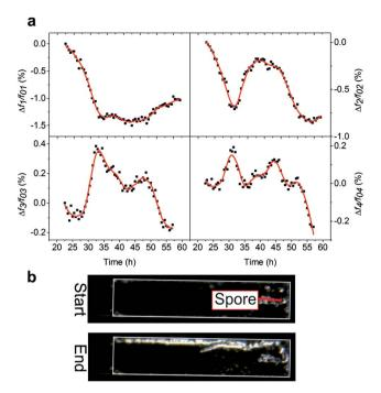
Fig. 3 Data concerning growth measurement performed using a 2  $\mu$ m thick cantilever. (a) Relative resonance frequency shifts due to *A. niger* growth for the first four resonance modes. (b) Images recorded at the start and end of the growth measurement. Hyphal growth has occurred along the left side of the cantilever. The cantilever outline is shown in white. Initial spore position is also indicated.
