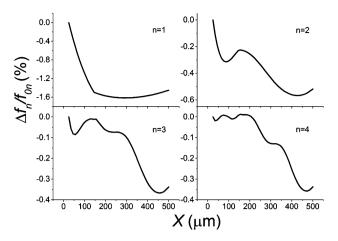
Fig. 6 FEM of hypha growth along the longitudinal axis of a 2  $\mu$ m thick cantilever. Similar trends to those measured experimentally are observed, however not at the same positions.
