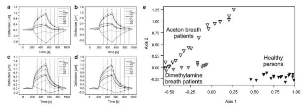
**Figure 5:** (a)-(b) Cantilever deflection traces acquired during injection of a breath sample of a healthy person, (c)-(d) *ditto*, but for a patient suffering from *uraemia*. (e) PCA plot.
