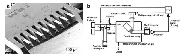
**Figure 1:** (a) Scanning electron microscopy picture of a microfabricated cantilever sensor array. (b) Schematic of the gas phase cantilever sensor array setup.
