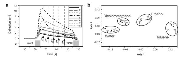
**Figure 2:** (a) Cantilever deflection traces during exposure of a polymer-coated cantilever array to dichloromethane vapor. (b) PCA plot demonstrating the recognition capability of the cantilever-array based artificial nose.
