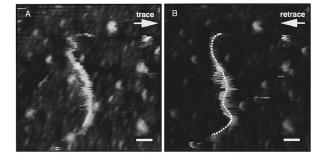
FIG. 5. SFM images of a thiol-modified 2249 bp DNA segment (length  $\approx$  750 nm), on bare TSG in propanol in dc mode. Simultaneously captured data set of the same segment, but with different scanning directions: (A) left- to right-hand side, and (B) right- to left-hand side; bars=100 nm (scan speed 1 Hz) (from Ref. 13).
