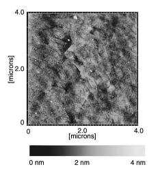
FIG. 1. DFM image of the DSU SAM on Au (111) taken in air in the noncontact mode.
