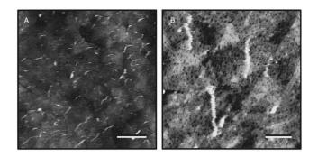
FIG. 4. DFM images of the amino-modified 806 bp DNA segments (length  $\approx 250$  nm), bound to a DSU SAM on Au(111), in 10 mM borate buffer (*p*H 9.0): (A) measured with the homebuilt DFM, bar=500 nm; (B) measured with Nanoscope III, bar=200 nm.
