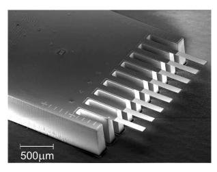
Figure 1. Scanning electron microscopy (SEM) image of the cantilever array.
