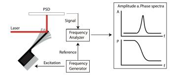
Figure 2. Measurement setup.
