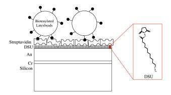
Figure 3. Schematic illustrating the binding of biotin latex beads immobilized on the streptavidin-functionalized cantilever surface.
