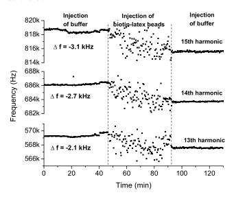
Figure 5. Frequency shifts due to biotin-streptavidin coupling of latex beads to the cantilever surface.
