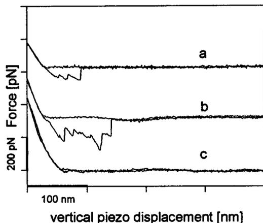
FIGURE 2 Typical approach/retract cycles taken between a BBSA-coated sensor and a ABIO-coated surface. The adhesion peaks are in the piconewton range and are often multiple (*curves a and b*) (discussion in text), whereas the BSA control (*curve c*) shows hardly any adhesion.
