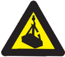
Beware, overhead load
