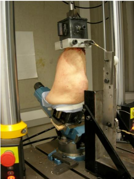
Peter O'Reilly explains 'we are looking at the effect on knee motion of using a new type of Anterior Cruciate ligament graft. The picture shows the knee upside down so that the tibia is uppermost and the femur below. The tibia is being displaced relative to the femur via a pulley arrangement using the third axis of the machine which is out of view. We are doing this at various angles of flexion which are set on the Universal vise which is gripping the femur.
