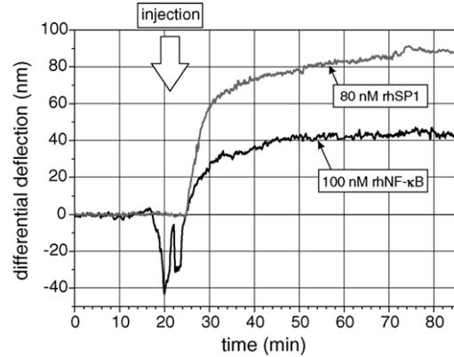
Fig. 5. Comparison of rhNF- $\kappa$ B with rhSP1. Differential signal of experiments conducted by injection of 100 nM rhNF- $\kappa$ B or 80 nM rhSP1 to two different cantilever arrays. For rhNF- $\kappa$ B, cantilevers functionalized with SP1-binding oligonucleotides were used as reference. Cantilevers functionalized with the rhNF- $\kappa$ B-binding oligonucleotides served as references when rhSP1 was injected.
