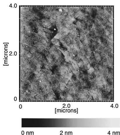
FIG. 1. DFM image of the DSU SAM on Au (111) taken in air in the noncontact mode.
