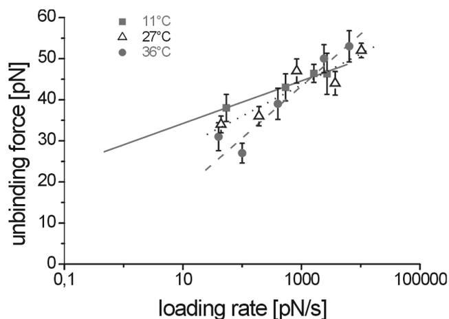
**Fig. 3.** The most probable unbinding force as a function the loading rate (*e*-tip/*f*-surface, 16 bp) obtained at different temperatures. Squares (11 °C), triangles (27 °C), circles (36 °C).
