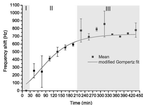
Fig. 3. Mean values of resonance frequency shifts due to bacterial growth of the sensor-cantilever of multiple measurements as a function of time. The shown curve corresponds to a modified Gompertz model fit (Baty and Delignette-Muller, 2004). Bacterial growth phases: (I) lag-phase; (II) exponential-phase; (III) stationary-phase. Bars correspond to the standard deviation.
