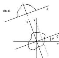
**FIGURE 6.19** CAT scan geometry. The path of a typical beam is shown by the dotted line; its attenuation is represented by a single point in the projection  $p(\xi, \phi)$ .
