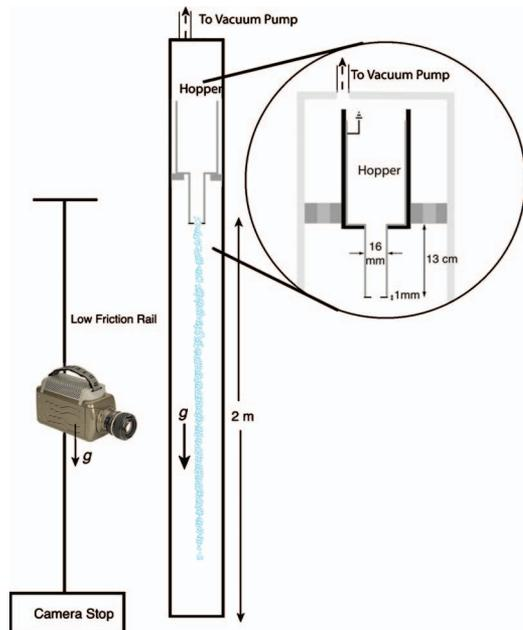
FIG. 1. (Color) Schematic of falling camera setup.
