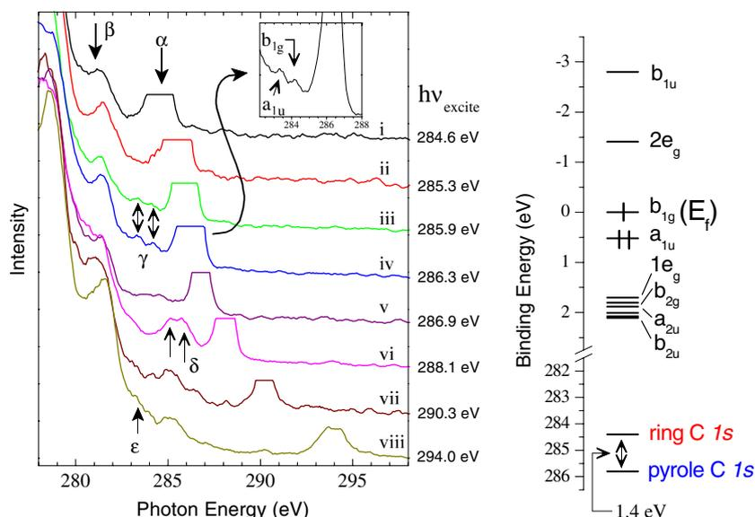
Fig. 2. Left panel: Series of SXE spectra from CuPc showing emission from states near  $E_F$ . Right panel: Electronic structure of CuPc near  $E_F$  as predicted by DFT calculations [3], with measured C 1s core level binding energies indicated. Note that the DFT calculation energies have been rigidly shifted such that the binding energy of the  $b_{1g}$  state at  $E_F$  is set to zero, allowing comparison to the measured XPS spectra and the excitation energies in the RSXE spectra.
