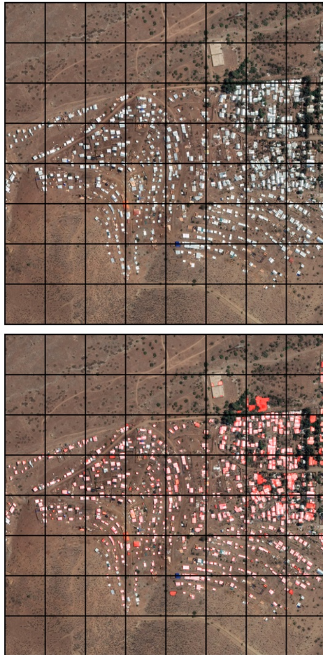
Figure B2: Example Predicted Building Footprints - Slum in Santiago Metropolitan Area a
