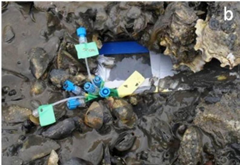
**Figure 13.** (a) Pore-water profiler with Rhizon™ soil moisture samplers placed at 0, 1, 2, 3, 4, 5, 8 and 10 cm intervals. (b) Pore-water profiler inserted into a mussel-bed.
