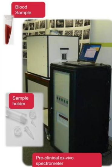
Figure 2: New detection equipment for quantitative analysis of MNP's in blood and tissue samples
