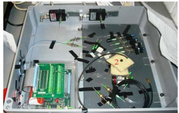
Picture of the prototype OSNR monitor built in TCD.
