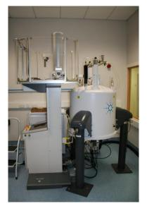
(<sup>1</sup>H), Carbon (<sup>13</sup>C) and Nitrogen (<sup>15</sup>N) for 2D and 3D structural NMR at very high signal to noise ratio. A second probe is optimised for 1D and 2D analysis for proton and nuclides from <sup>109</sup>Ag to <sup>31</sup>P. This is a NMR spectrometer designed for protein NMR and research synthetic chemistry programs
