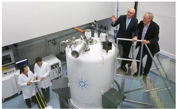
The system is equipped with a number of different probes, including a cryogenically cooled triple resonance ColdProbe which provides significant sensitivity gains and is ideal for low concentration samples in either non-ionic or highly ionic solvents. The 800 MHz ASC (Actively Shielded Compact) magnet draws on the latest super conducting wire technology to make this super compact shielded magnet which operates at a temperature of 4.2 Kelvin (K). The NMR has a 12 station auto-loader.
