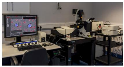
to 8 wavelengths simultaneously between 470nm and 670nm. It has an inverted microscope with 10x and 20X dry objectives and 40X, 63X and 100X oil objectives. It also has a resonant scanner for imaging at 24 frames per second and 37 degree incubator. This microscope has both high resolution and flexibility to cover a wide range of experimental setups in fluorescent microscopy.
