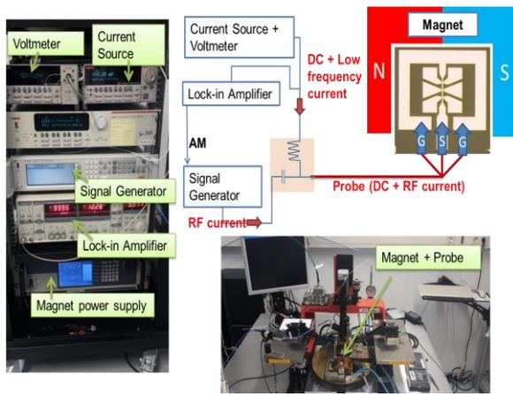
All samples were patterned into Hall bars using the UV photolithography facilities available at HZDR. The contact pads were designed to allow the connection of high frequency ground-signal-ground (GSG) probes to the sample. All samples were patterned successfully and showed the same magnetoresistive response as the extended films. ED-FMR experiments were performed on samples with different structures in the setup shown here. More details can be found in [1].
