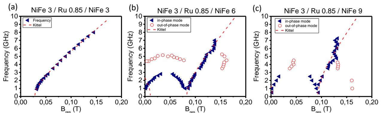
**Figure 2: Fitted resonance peaks from electrically detected magnetic resonance for the balanced (a), slightly unbalanced (b), and very unbalanced (c) artificial ferrimagnets. In the fully balanced system the out-of-phase mode is most difficult to detect as the contribution to the change in resistance of each layer is effectively cancelled.**
