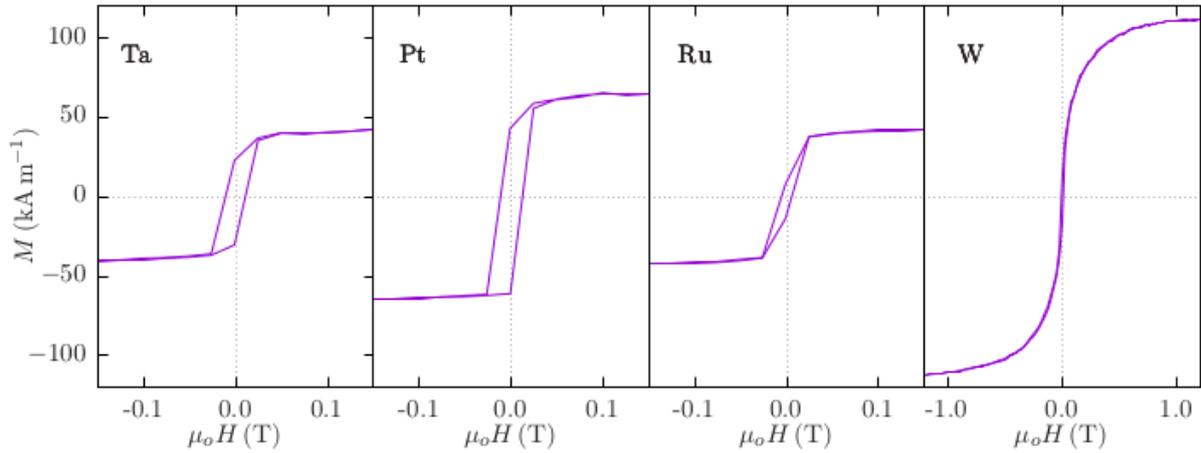
Figure 5 – Out-of-plane SQUID magnetisation loops taken of GdFeCo on various seed layers
