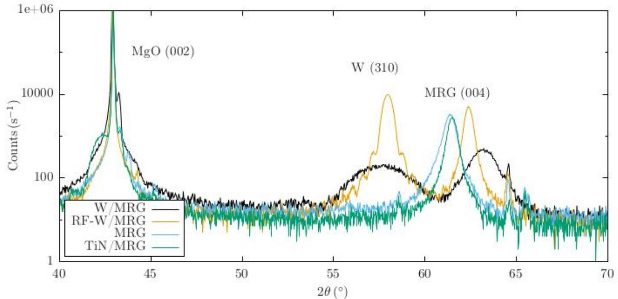
Figure 1 - XRD of MRG grown directly onto substrate versus different seeds. Substrate is always MgO
