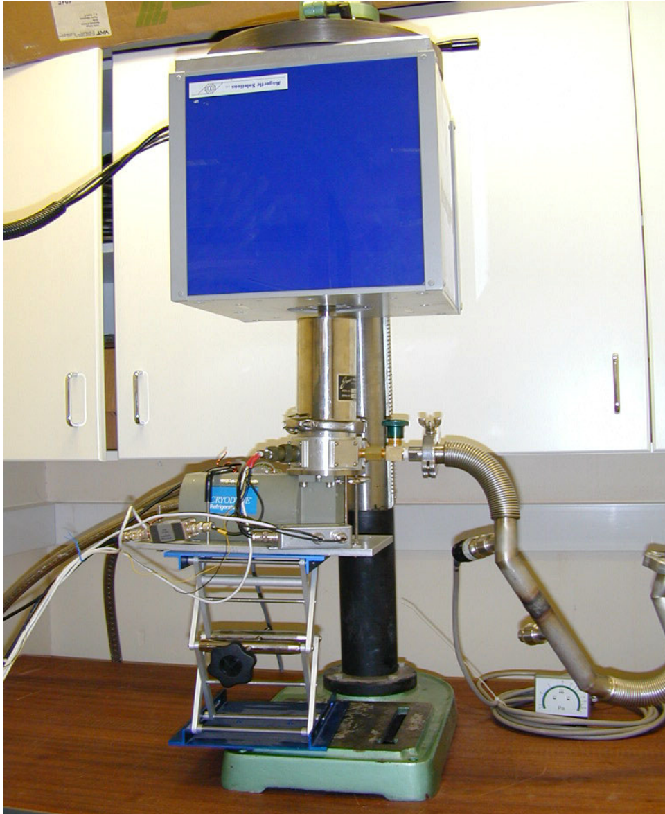
Figure 3.8: Photograph of the CCR system in MR measurement configuration. The measurement head is inserted into the permanent magnet.
