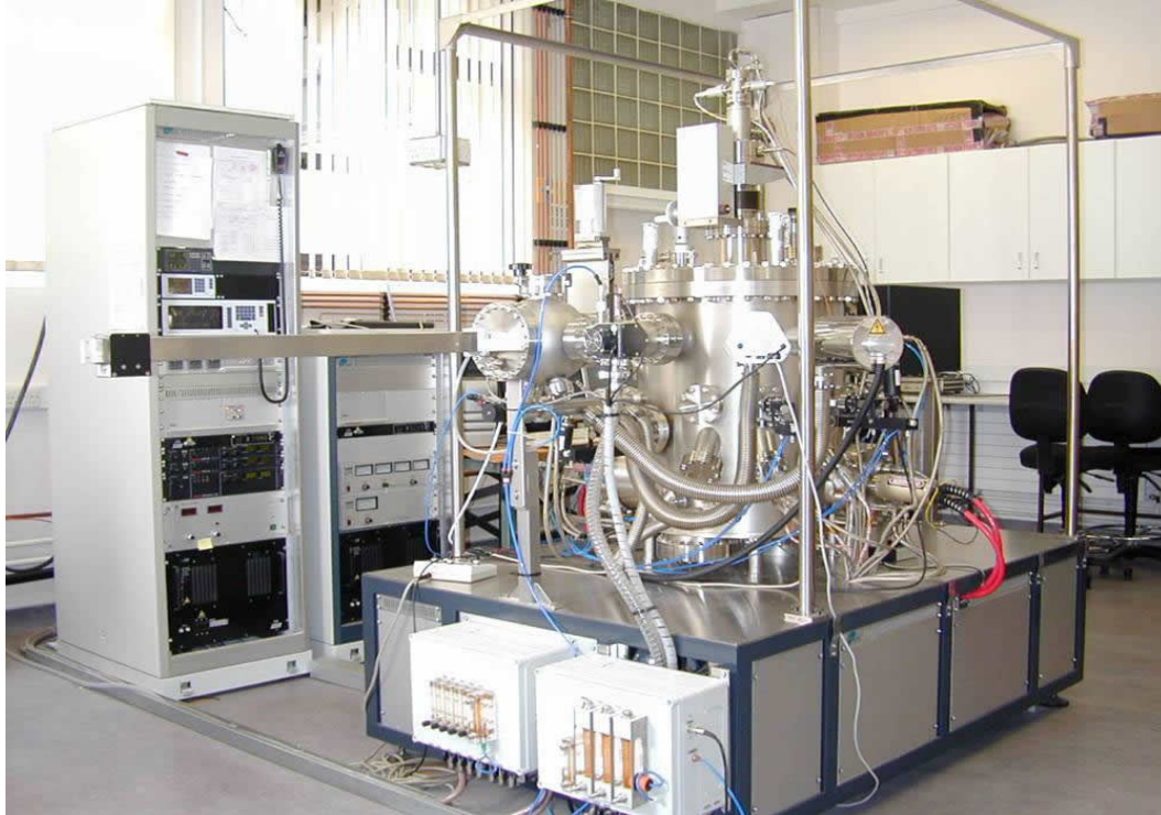
Figure 3.1: The entire MBE system, including the load-lock chamber, the deposition chamber, the transfer arm and the assorted power electronics cabinets.
