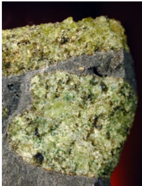
Figure 2: The green patches are a xenoliths of the rock-type peridotite, which makes up the uppermost mantle. The xenoliths are encased in dark grey basalt, an igneous rock formed by partial melting of peridotite.
